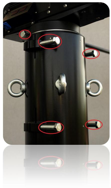
After those steps the inner column can be raised or lowered with a 24mm ratchet or by using the drill. The column can be extended by 45cm until visible marking appear.
