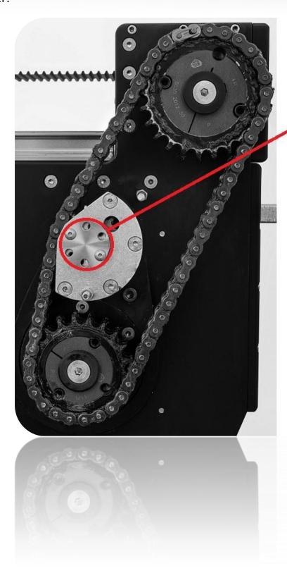
Stretch the chain using this tensor. Chain can't be stretched too much. After - attach the screws that were released before.
