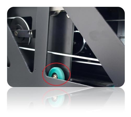
To tune up the green wheel you need to loose (don't release it) the helical screw...
