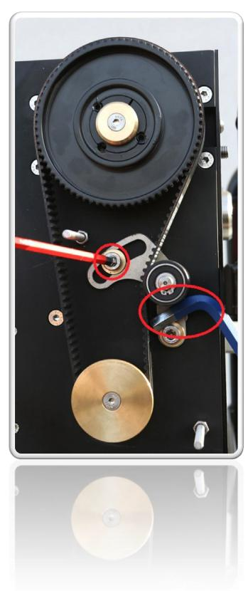
4. Remove the blue key and tighten the screw.
