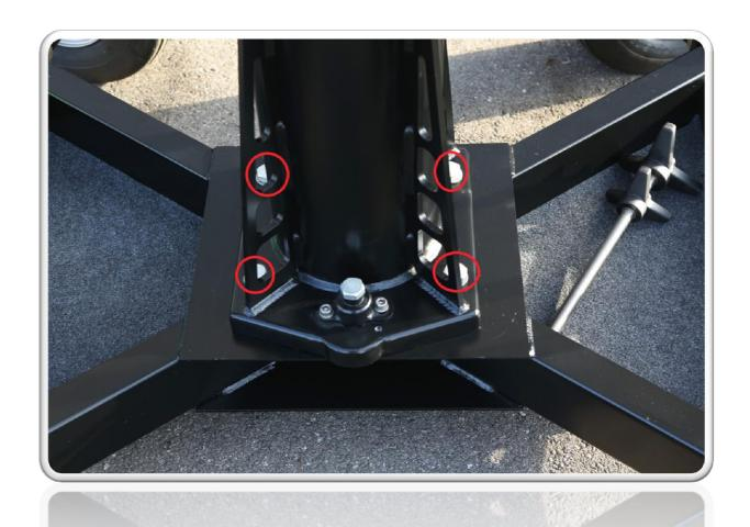
**C.2.** The column can be raised by 45cm (until visible mark appears). There are 4 screws that needs to be released before extending telescopic column and also horizontal break must be locked. After those steps the column can be raised or lowered with a 24mm ratchet or by using the drill.
