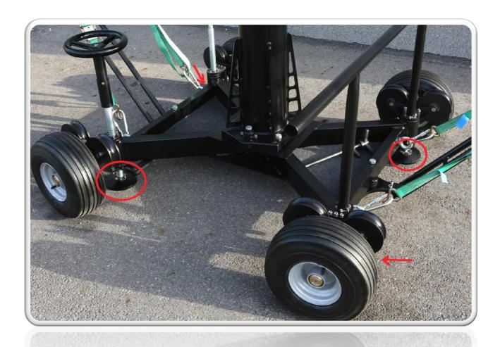
**D.2.** Track wheels are also permanently attached into the dolly (1m width).
