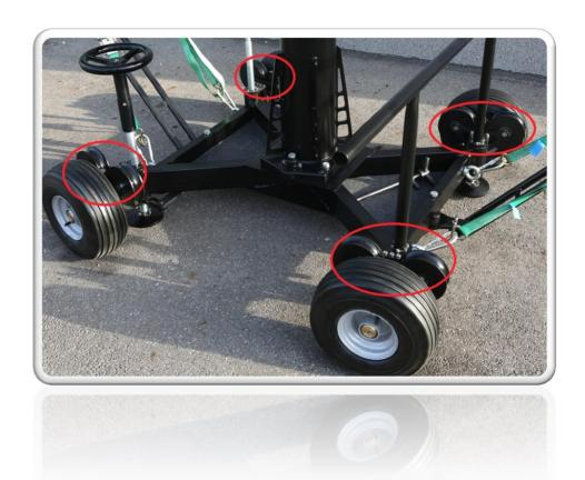
**D.3.** On the dolly there's a steering supported by 2 drawbacks connected to each other for best maneuvering of the crane. Optionally it's possible to block one of the drawback and separate it from the other one by dismounting the connecting strip under the dolly.
