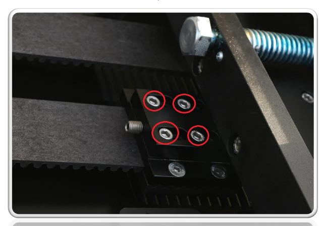
3. Tighten the belt using the screw. After tight the screws you loosened up before.
