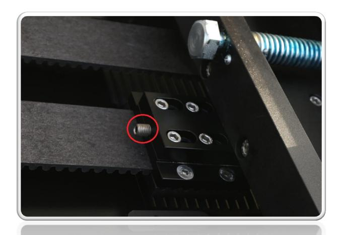
4. Operation should be performer on both sides of the platform to evenly tighten the belt.
