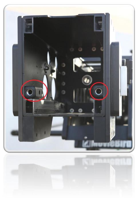
2. Put the extension into section so the screw will fit into the hole. Then we screw the nut tightly so there won't be any loose on the extension.
